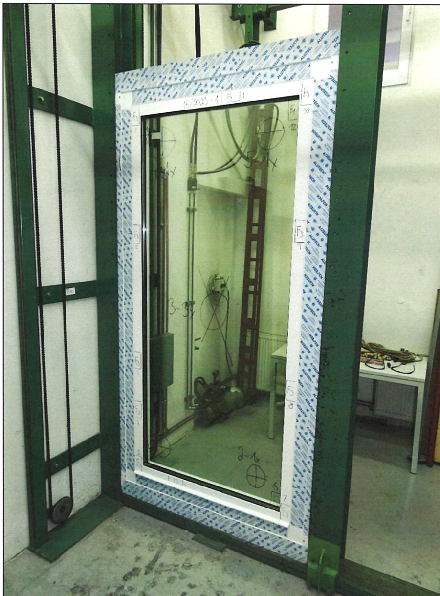
Pic. 9 – test sample No. 15/2023-1 after static and dynamic tests
