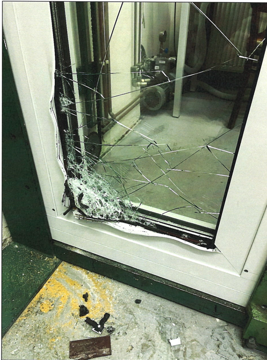
Pic. 16 – test sample No. 15/2023-2 after manual test No. 6 (view from the side of the attack – outside)
