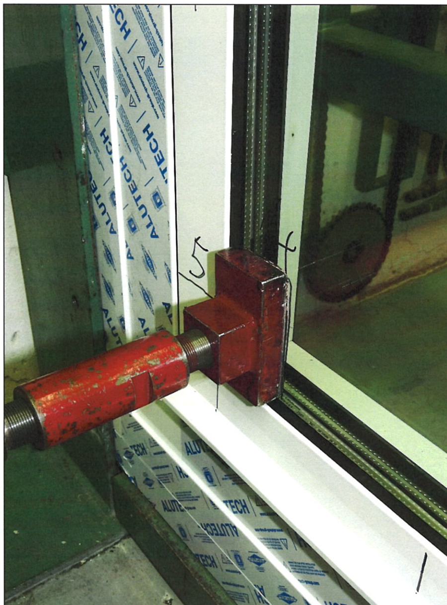
Pic. 7 – detail of point No. 14 during a static loading test, test sample No. 15/2023-1
