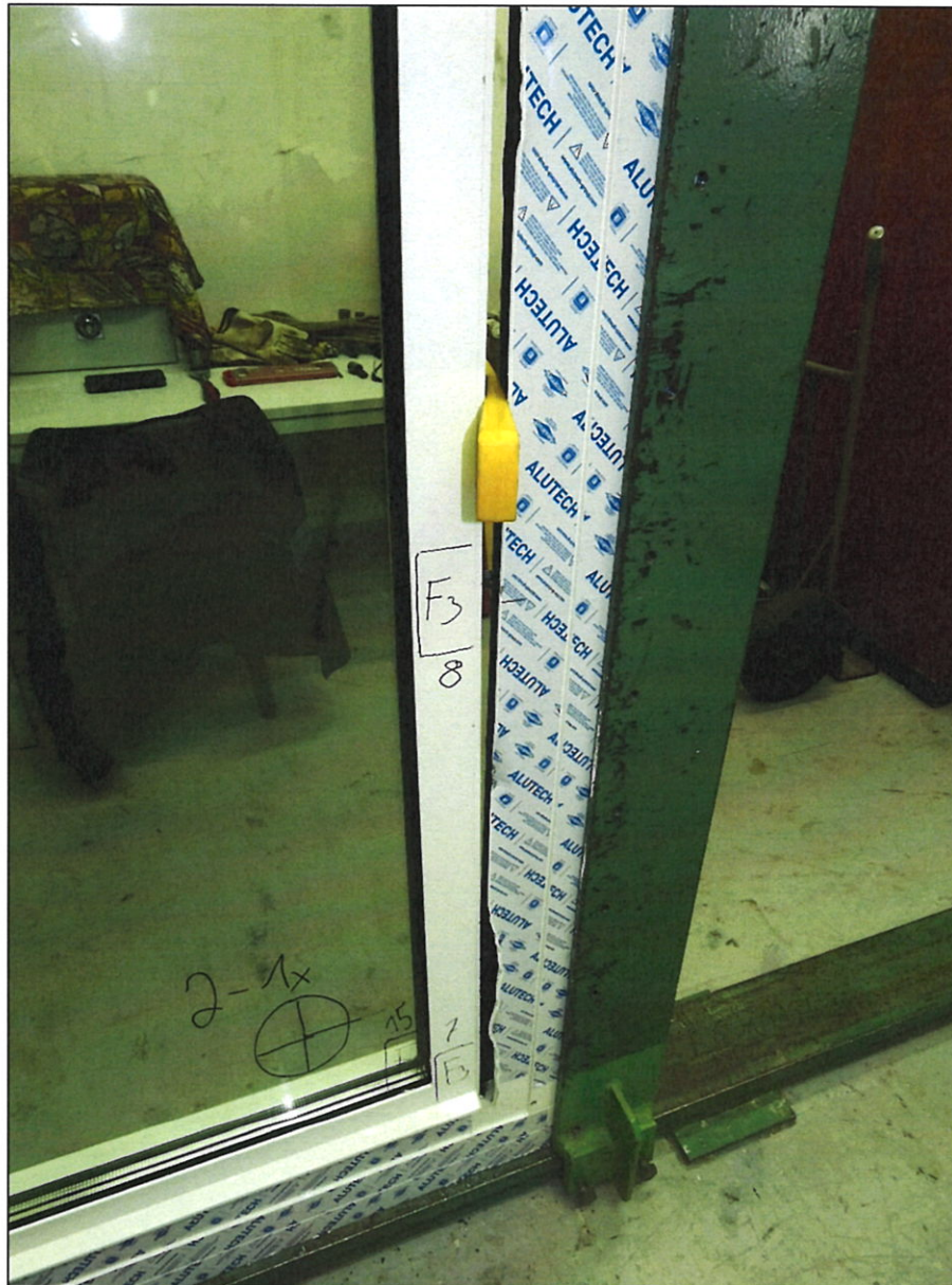
Pic. 10 – test sample No. 15/2023-1 after manual test No. 3 (view from the side of the attack – outside)
