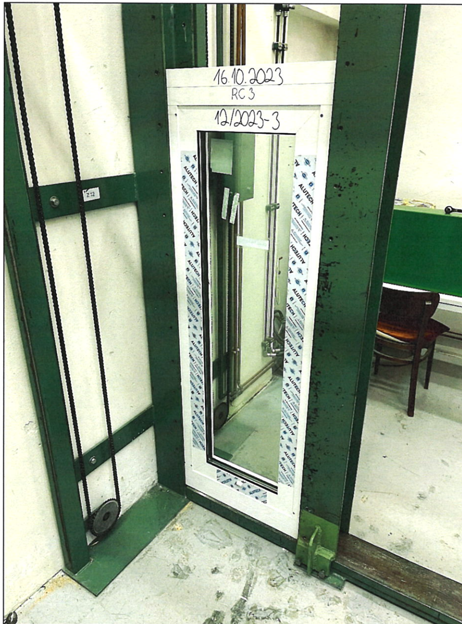
Pic. 14 – test sample No. 12/2023-3, Thermal brake one leaf window type W72 – RC 3
