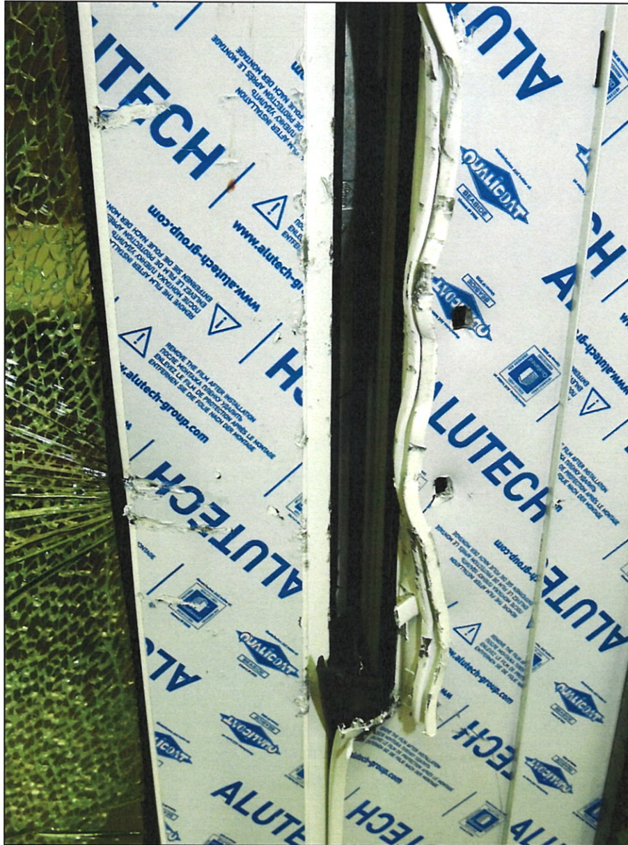
Pic. 13 – test sample No. 12/2023-2 after manual test No. 6 (view from the protected side – outside)
