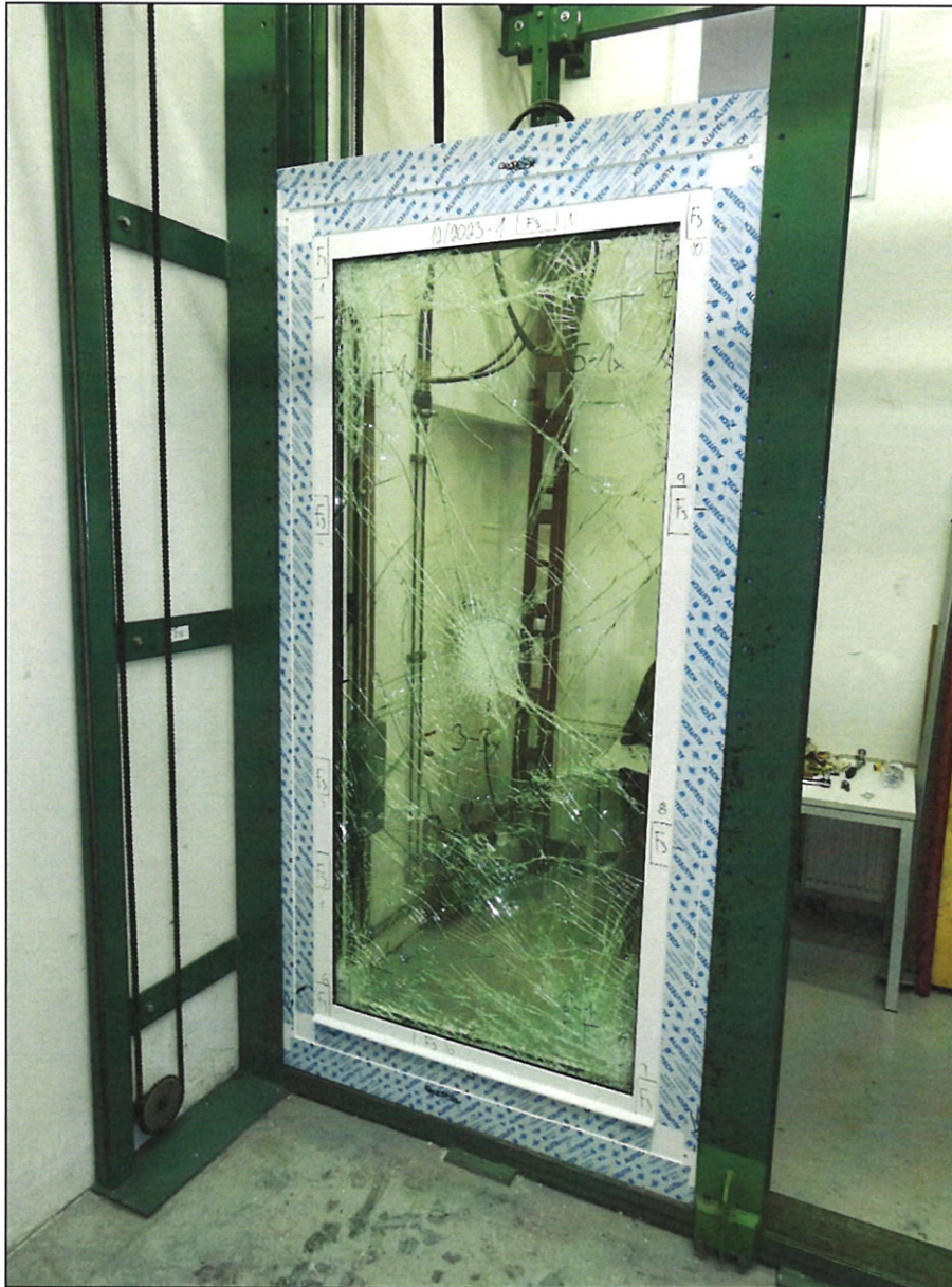
Pic. 9 – test sample No. 12/2023-1 after static and dynamic tests
