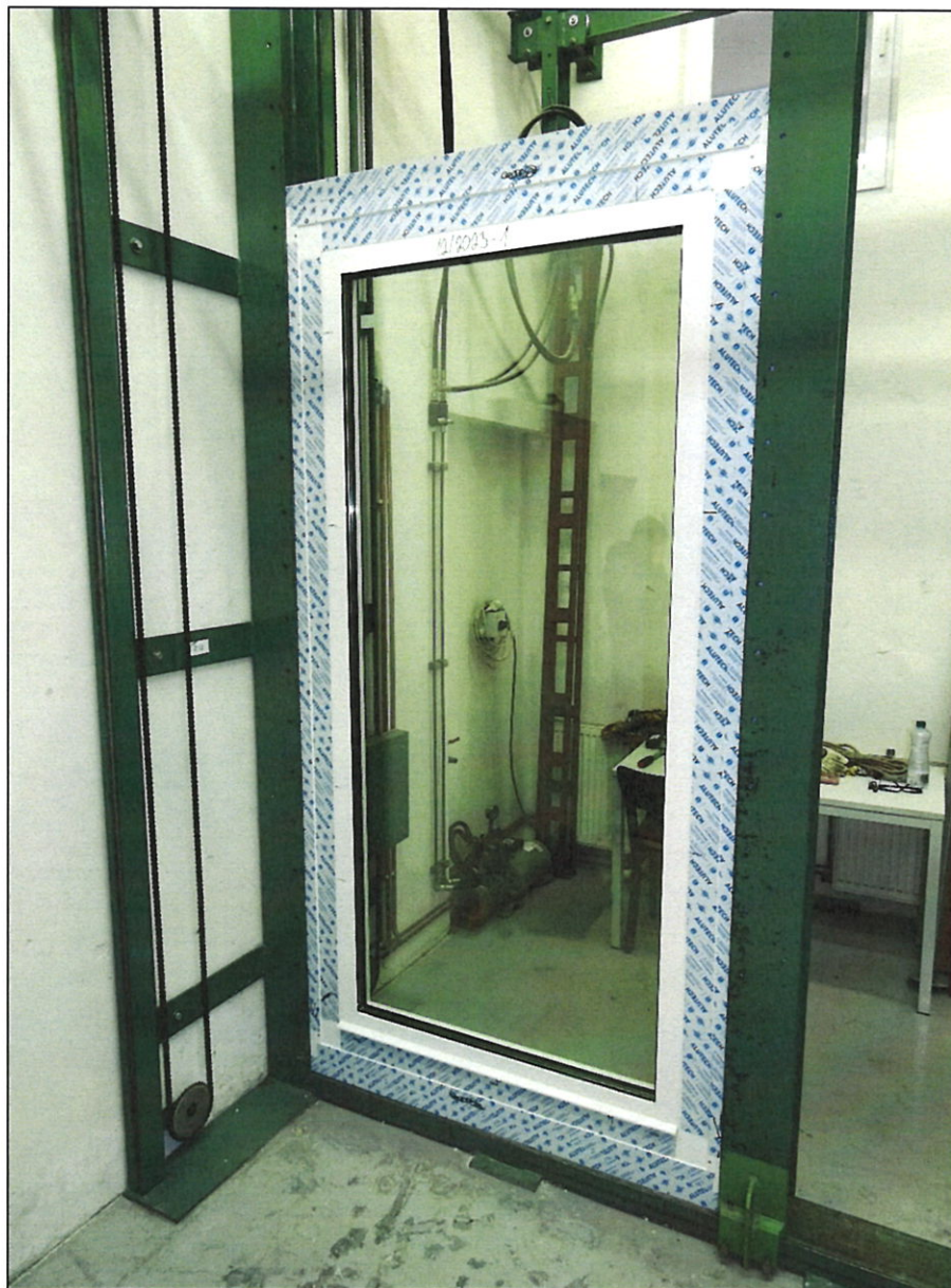
Pic. 1 – test sample No. 12/2023-1, Thermal brake one leaf window type W72 – RC 3
