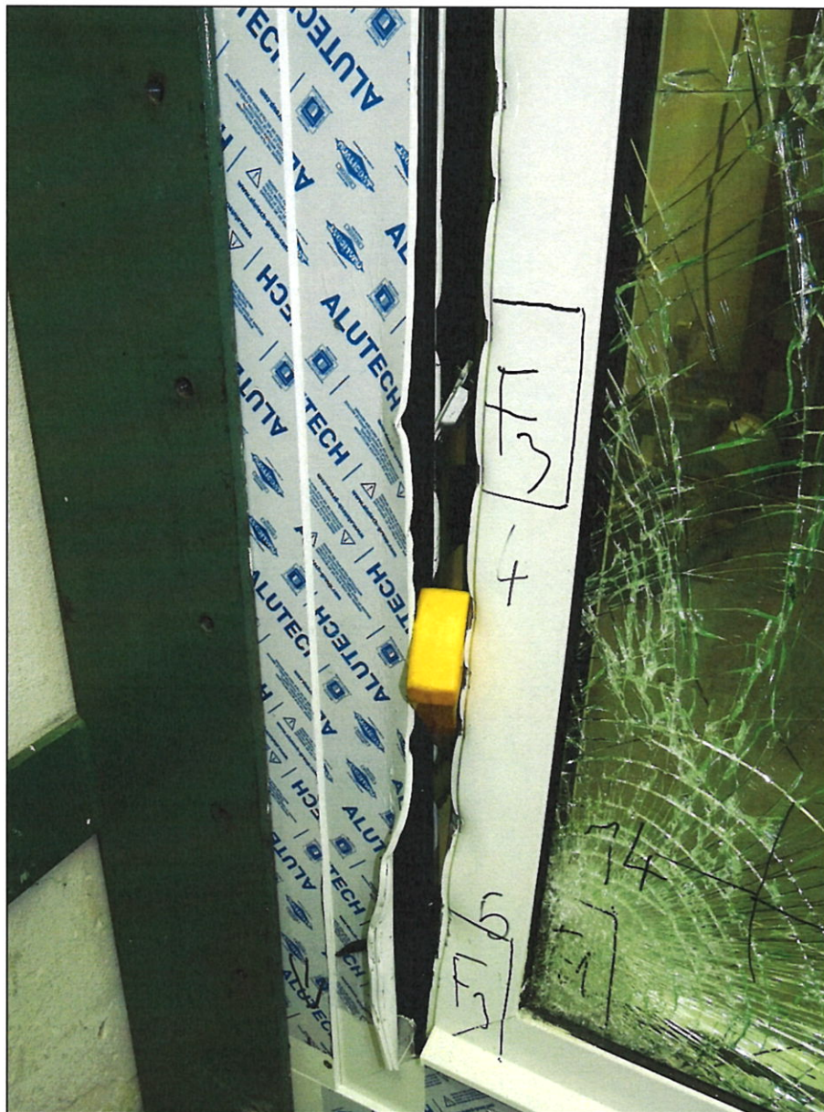
Pic. 11 – test sample No. 12/2023-1 after manual test No. 4 (view from the side of the attack – outside)
