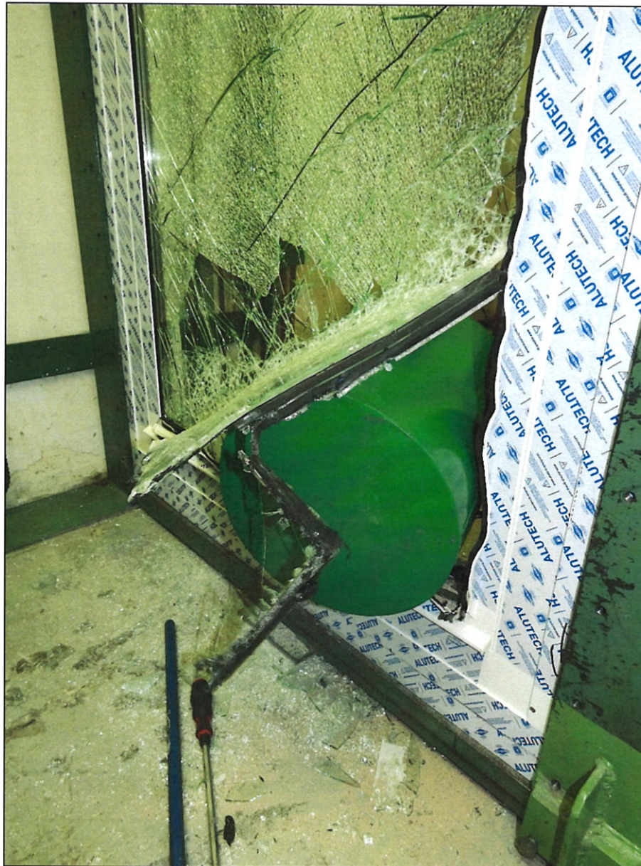
Pic. 12 – test sample No. 12/2023-2 after manual test No. 5 (view from the protected side – outside)
